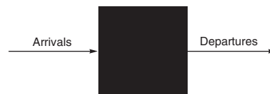
Figure 6.15 Treating the I/O system as a black box. This leads to a simple but important observation: If the system is in steady state, then the number of tasks entering the system must equal the number of tasks leaving the system. This flow-balanced state is necessary but not sufficient for steady state. If the system has been observed or measured for a sufficiently long time and mean waiting times stabilize, then we say that the system has reached steady state.
