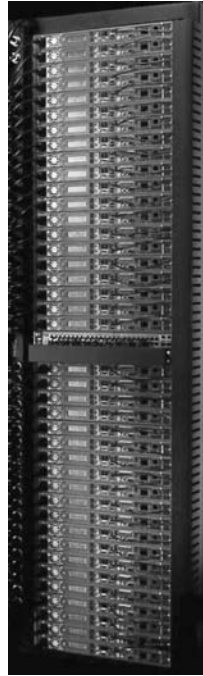
Figure 6.19 The TB-80 VME rack from Capricorn Systems used by the Internet Archive. All cables, switches, and displays are accessible from the front side, and so the back side is only used for airflow. This allows two racks to be placed back-to-back, which reduces the floor space demands in machine rooms.
